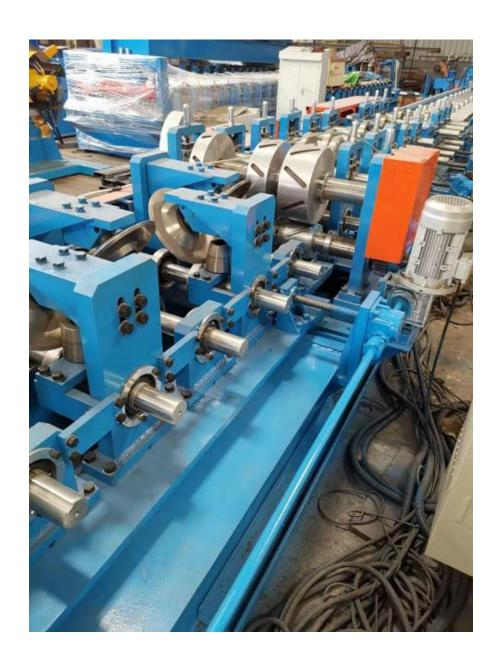
Formed Difference width, different height, different length C channel steel products.
