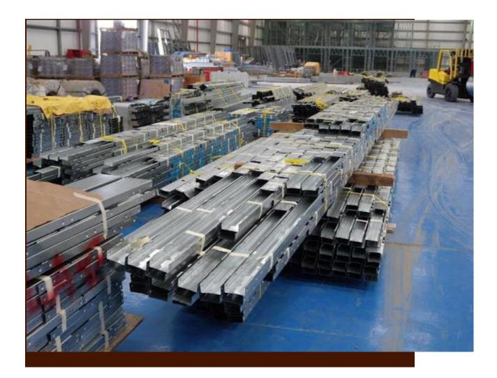
The Anti-seismic performance of light steel structures is better superior from traditional concrete and brick-concrete building homes. At the same time, since the structure of the light steel structure is light in weight and the weight per unit area is only 1/4 of the weight of the brick-concrete structure of the same area, the basic treatment is simple and suitable for most geological conditions. Steel-framed
