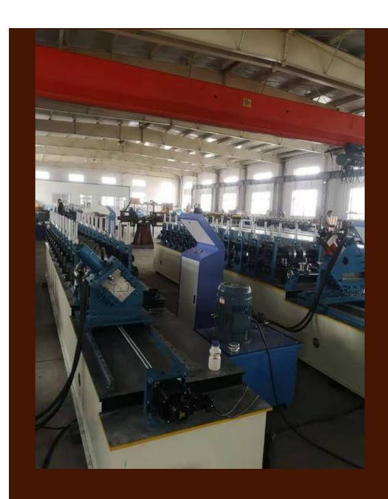
Light steel profiles made by roll forming machine process, such as u channel, c channel etc steel parts for building structure frame.
