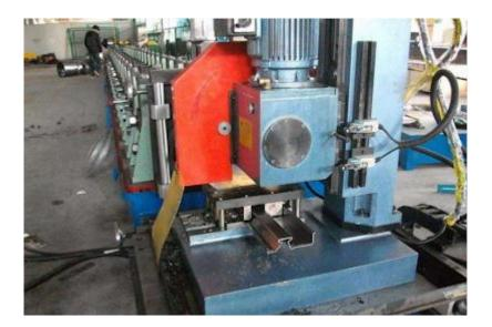
Cold bending machine debugging & Roll forming machine running testing
