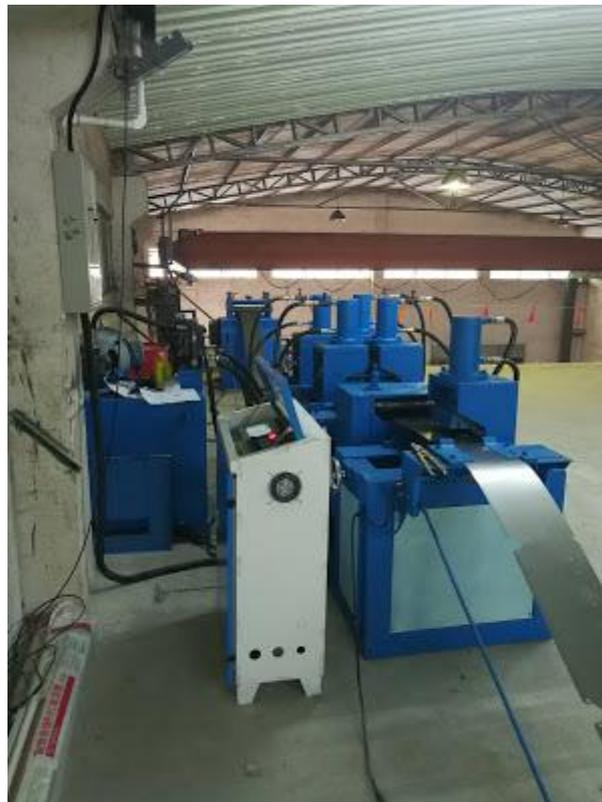
4. Roll forming machine system, The main machine base of this production line is welded with 100\*100\*3MM square steel, Shenzhen Superda
