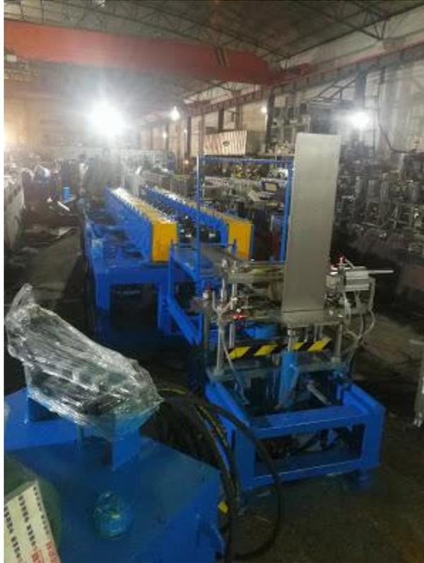
C: Transmission part: It is the conveying part of the forming power of the production line. Its power is transmitted from the main motor to the reduction gearbox, and then the gearbox is transmitted to the driving wheel through the gear. The driving wheel passes the excessive gear transmission, so that the upper and lower rolling turns synchronously.
